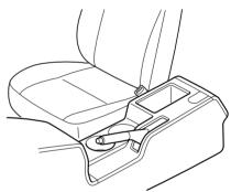
Small items can be placed in the tray of the center console lid. To open it, pull the right release latch.
